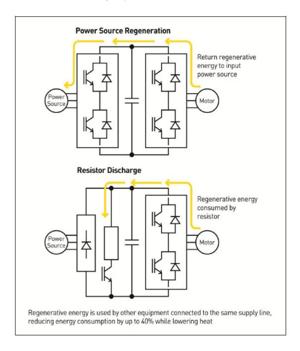
Power source regeneration requires a drive system with an intelligent power module that can sense the flow of current and switch accordingly. When used, the effects are significant. Implementing a servo driven system utilizing drive amplifiers with power source regeneration can see a savings of 30% to 40% in electrical power consumption.
