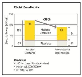
Pulse width modulated (PWM) amplifiers provide an excellent control method for electric motors in automation equipment. Rapid acceleration with precise speed and current control is possible but there are always switching losses when using a PWM drive system. These losses translate into waste heat generation. Using the latest generation of power devices will increase controllability and reduce the heat loss. Reduction in heat loss directly equates to electrical energy savings.
